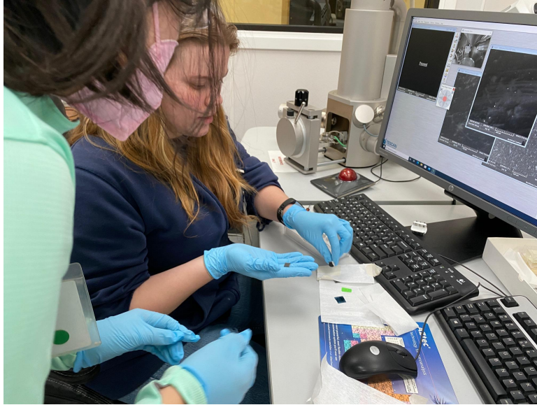
Imaging samples that were already coated with DLC under a scanning electron microscope (SEM) to observe the tip morphologies of the DLC.
