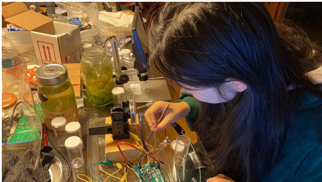
Using the microgram scale made from a repurposed galvanometer to measure the weights of various plastic particles
